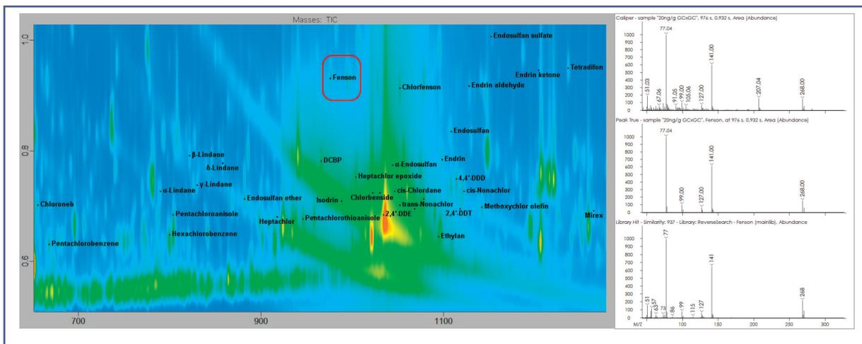
**Figure 1. Section of Contour Plot of the spinach QuEChERS extract with dSPE cleanup (left) spiked with pesticides at 20 ng/g. The improvement in chromatographic separation with GC×GC significantly improves both peak detection and quantification. In this example, the second dimension of separation effectively moved the pesticide Fenson away from large matrix interferences.**
