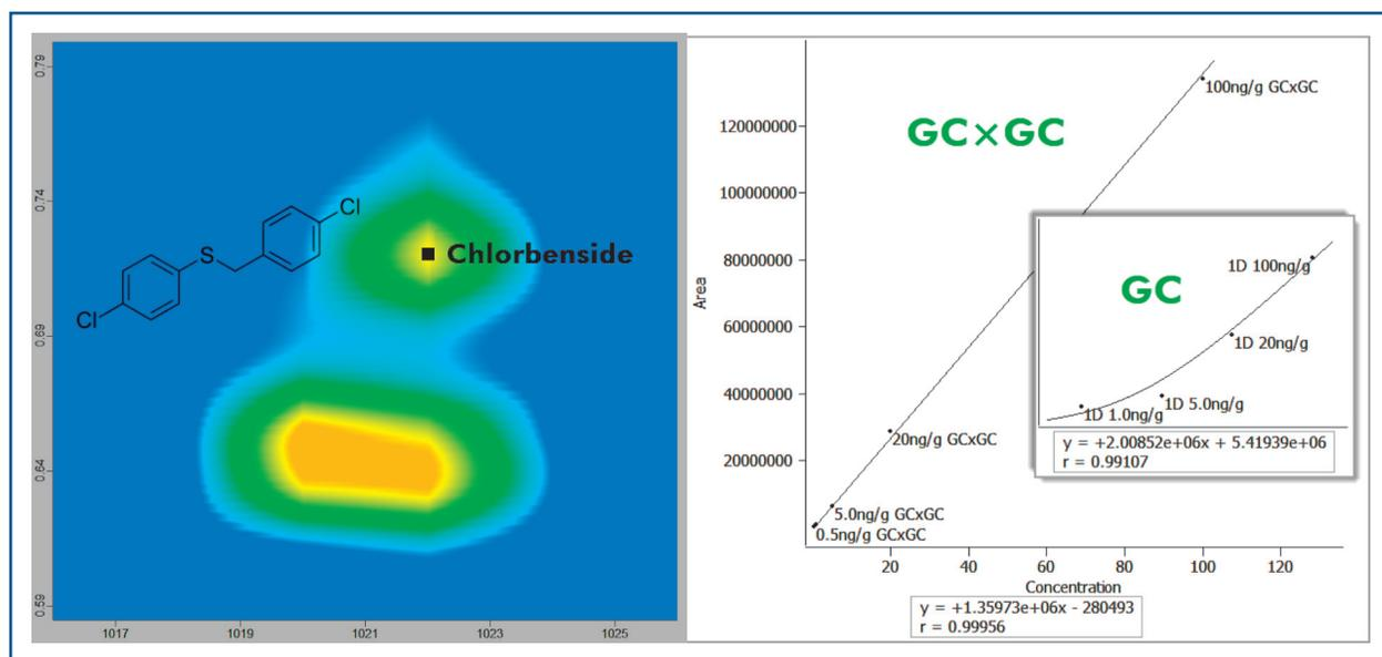
**Figure 4. GC×GC resolution of Chlorbenside from the matrix interference. The GC×GC separation allows for a linear and sensitive quantitation curve. In the GC separation, the coeluting matrix completely obscures the pesticide below 20 ng/g making consistent, accurate integration impossible.**
