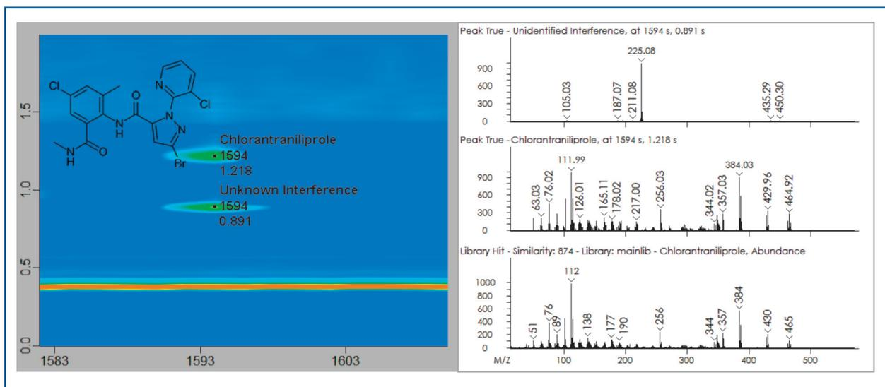
**Figure 7. GCxGC Contour & Spectral plots of Chlorantraniliprole and the interference compound. The two compound signals have been normalized to allow for easier viewing. Note the separation from the column bleed (horizontal band) and the improvement in the deconvolution of both compound spectra compared to their GC results in Figure 6.**
