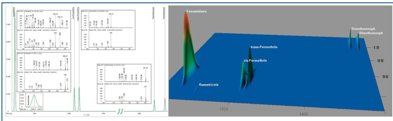
Figure 5. Initially identified incurred pesticides and plasticizer (Bumetrizole) shown in both GC Chromatograms and GC×GC Surface Plot.
